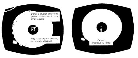
Figure 4. Using SUPERSIGHT to locate the center of a part to sub-pixel accuracy.
